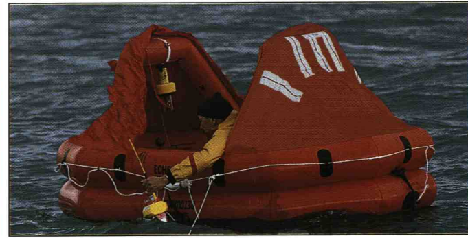
Loud beeping indicates to survivors that the 9 GHz transmission has been received by the radar of vessels and aircraft in the area.
