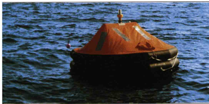
Liferaft fitted with RESCUER SART and KANNAD Epirb in operation after release from float free container
